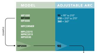
Note: MP Rotators are designed to operate in conjunction with a pop-up sprinkler or shrub sprinkler. Also compatible with G-Spray (see following page).
