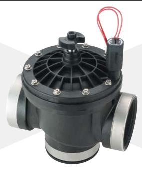
fabric-reinforced diaphragm and flow control as standard. It withstands pressures of up to 220 PSI (15 bars) as it effortlessly handles relentless water hammer. And with the Accu-Set option as a pressure regulator, it maintains the safest, most constant water pressure level.
